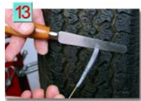
13. After inflating, cut the plug flush with the outside tread area. Return tire to service.
