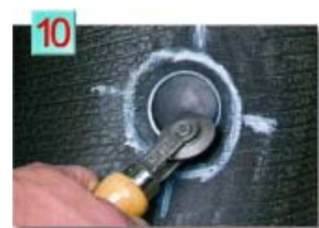
10. Stitch the repair unit vigorously from the center working outwardly. Use as much hand pressure as possible.
