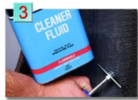
3. Clean the area around the injury with Patch Rubber Cleaner Fluid and a scraper.
