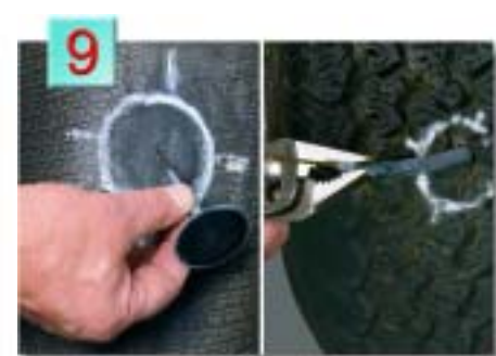
9. While the cement is still wet, insert the guide wire through the injury from the inside. Using pliers, grasp stem behind the wire and pull until the patch is seated against the innerliner. Do not over-pull and cause the patch to dimple. DO NOT USE PILOT WIRE TO PULL STEM THROUGH.
