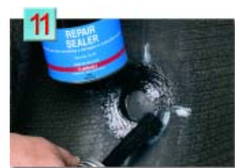
11. Apply Patch Rubber Repair Sealer to the over buff area.
