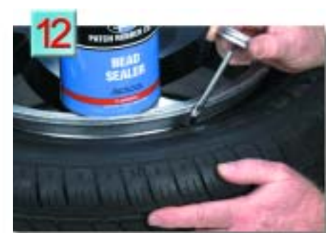
12. Apply Patch Rubber Bead Sealer to the bead of the tire before inflation to help prevent air loss around the bead.
