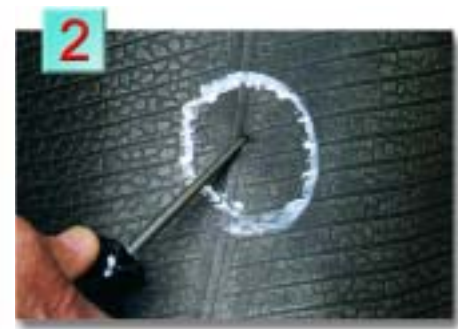
2. Remove foreign object and probe the injury with a blunt awl to determine the angle of penetration* *NOTE: IF THE ANGLE IS MORE THAN 20° FROM PERPENDICULAR, DO NOT USE THE COMBINATION PATCH-PLUG. USE A SEPARATE PLUG STEM AND THE APPROPRIATE REPAIR UNIT.
