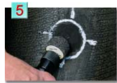
5. Use a low speed buffer (max. 2500 RPM) and a buffing stone to buff the innerliner 1/2" larger than the patch (RMA #1 Buffing Texture.) BE CAREFUL NOT TO BUFF THROUGH THE INNERLINER.
