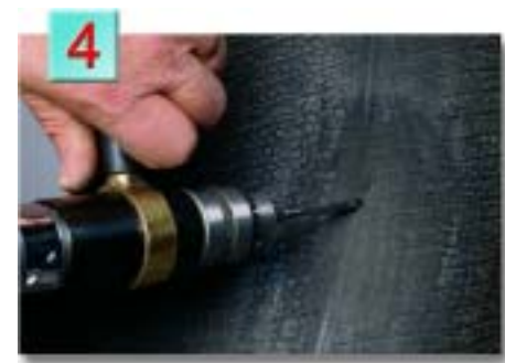
4. Using a low speed drill (500-700 RPM) and the appropriate size carbide cutter*, ream the injury following the angle of penetration four times from the inside of the tire, and four times from the outside. *REFER TO CARBIDE CUTTERS BELOW.
