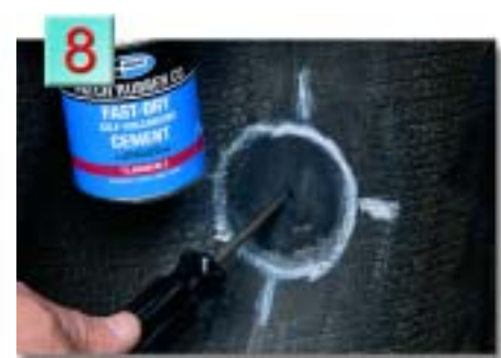
8. Dip awl into cement and insert into injury to lubricate the injury. DO NOT ALLOW TO DRY. DO NOT DRIP CEMENT ONTO BUFFED AREA.
