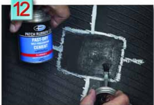
**12.** Apply an even coat of Patch Rubber Fast-Dry Self-Vulcanizing Cement to the entire buffed area. Allow cement to dry until tacky. Never use blow dryers, compressed air, or heat lamps to facilitate drying. Drying time is affected by temperature and humidity.
