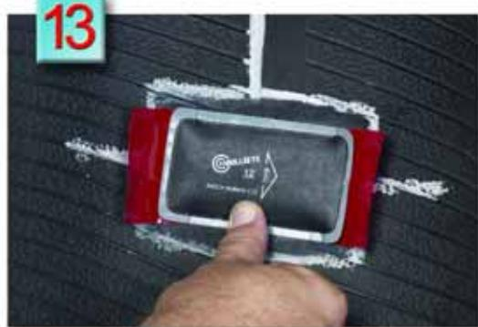
**13.** When cement is dry, partially remove the poly backing from the patch leaving just enough to hold the patch. Do not touch the back of the patch. With the beads of the tire in the relaxed position, apply the patch to the buffed area making sure the bead arrow points to the bead. Remove the remaining poly from under the patch.
