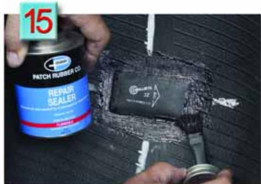
**15.** Apply Patch Rubber Repair Sealer to the overbuff area .
