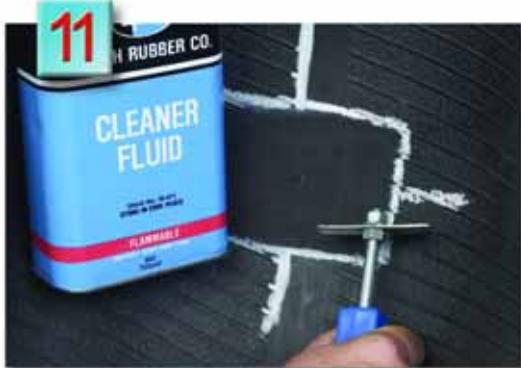
**11.** Apply a light coat of Patch Rubber Cleaner Fluid to the buffed area, scrape clean and allow to dry.
