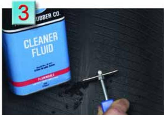
2. Remove the foreign object and probe the injury with an awl to determine the angle of penetration.
