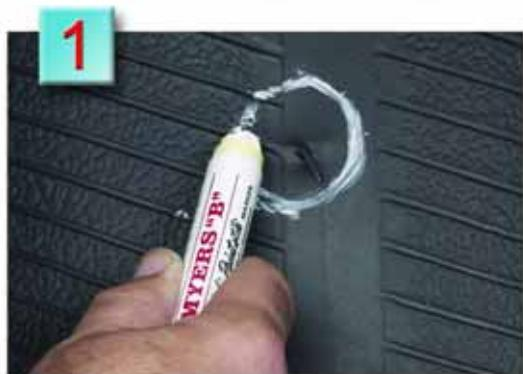
1. Locate the injury and circle with a tire crayon. **Consult warning on back cover for repairability of tires.** DO NOT INVERT RADIAL TIRES.
