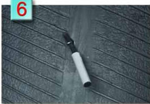
**6.** While the cement is still wet, push the wire puller through the injury from the inside of the tire. Grasping the wire, use a steady pull until 1/2" of the gray rubber on the plug is exposed outside the tire.
