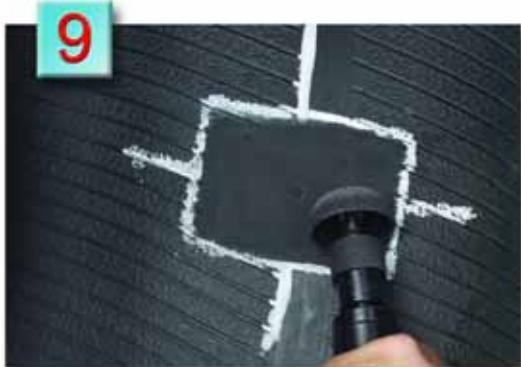
**9.** Use a low speed buffer (max. 5,000 RPM) and a buffering rasp to buff the plug and the outlined innerliner area (RMA #1 Buffing Texture). BE CAREFUL NOT TO BUFF THROUGH THE INNERLINER.
