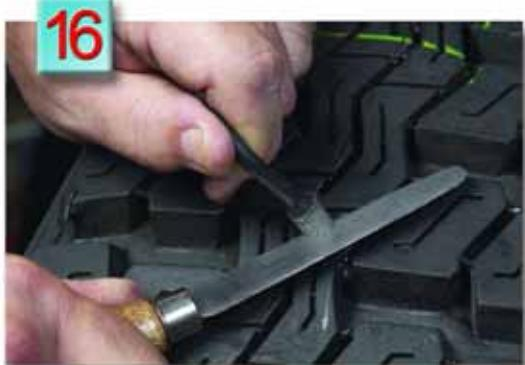
**16.** After inflating, cut plug flush with the outside tread area. Return tire to service.
