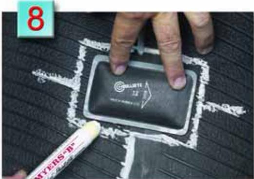
**8.** Making sure the bead arrows of the repair unit are pointing to the beads, center the repair unit over the injury. Use a tire crayon and outline an area 1/2" larger than the repair unit.
