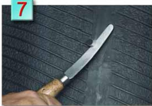
**7.** Using a flexible knife, cut the plug on the inside of the tire 1/8" above the innerliner. Be careful not to stretch the plug when cutting.
