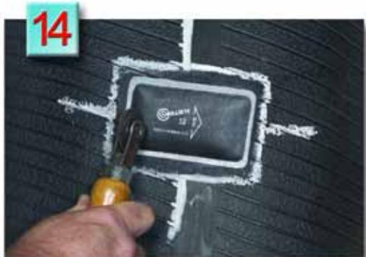
**14.** Stitch the repair unit vigorously from the center working outwardly. Use as much hand pressure as possible. Remove top cover film.
